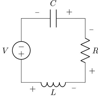
Figure 2.8: A driven RLC circuit.
