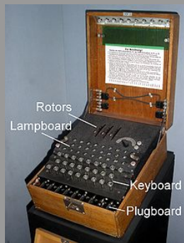
Figure: One of many military-enhanced Enigma designs, equipped with extra rotors and a plugboard.
