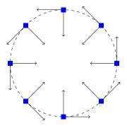
• An object moves with speed v around a circle of radius r
